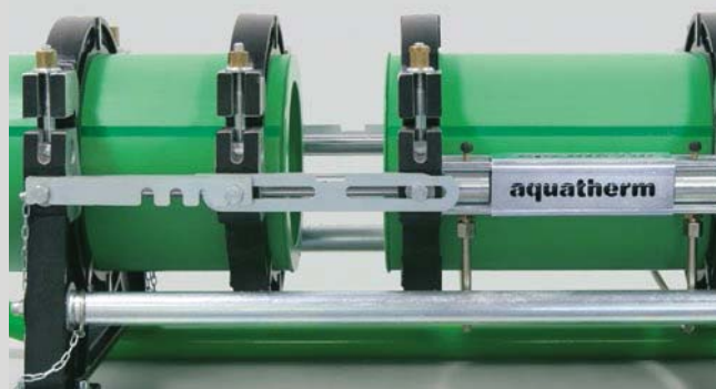
Divide the machine slide, remove heating element
