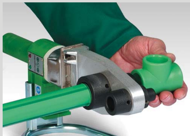
Heating-up of pipe and fitting
