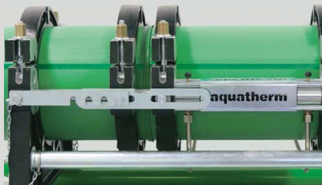
Join the pipes, cool down under pressure
