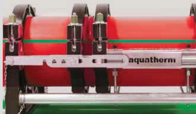
Join the pipes, cool down under pressure
