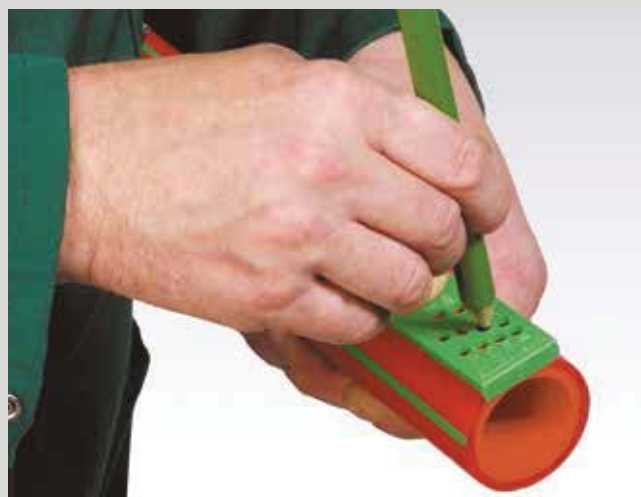
Marking of the welding depth
