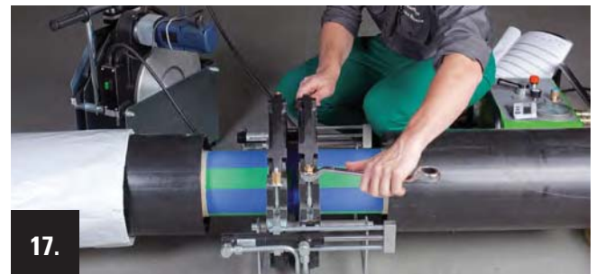
After the end of the cooling period the pressure is released at the hydraulic system. Then the mounting clamps are disconnected and the clamping device is removed.
